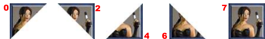
FIG. 17 - The purpose of shape is to define the shape of the texture sample and how it relates to the polygon's shape . The red numbers above mark the anchor corner of the texture sample for each texture shape.
