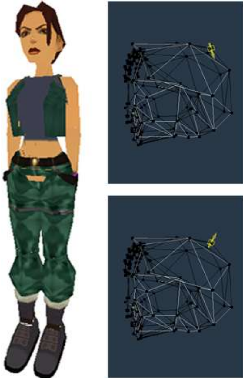
FIG. 13 - The normal vectors in the head of this custom model are not correct (top insert). They need to be recalculated, which can be done with STRPIX3.95R11 (bottom insert). (custom wad by L.Croft - AOD Louvre - from Lara's Level Base).
